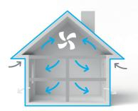
For homes with loft spaces, the PPS/L/H or PPS/L is installed in the loft and the discreet diffuser is installed in the hallway. For homes without loft spaces, the PPS/W/H is installed on the wall in a central hallway. Gently introducing tempered\* air into the house curing even stubborn condensation and issues.
